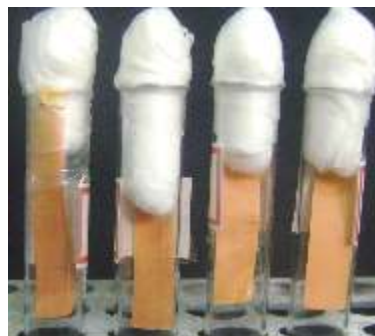
Figure 2. Color change of filter papers indicating the detection of HCN production
